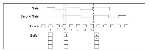
Figure 2-31. Buffered Two-Signal Edge Separation Measurement
